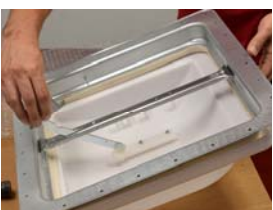
SLIDE CRANK ARM THROUGH BRACKET AND ATTACH TO LID
