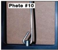
8) Using a pair of pliers, bend the end of the cable wire to form a loop around the end of the valve shaft. See photos # 9 and # 10.
