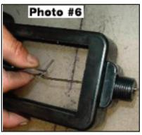
5) Insert the 90 degree bend into the hole of the valve shaft. See photos # 5 and # 6.
